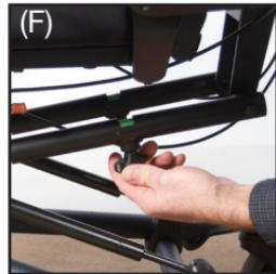
**Caution:** Make sure to have one hand supporting the back assembly, flipping the red plunger lever will cause the back assembly to fall.
