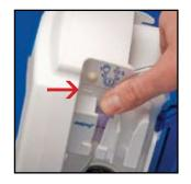
Grasp thumb tab on valve and insert ring retainer directly into left pocket. Press down on thumb tab to ensure valve is fully seated. Thumb tab must align with white line on left.
