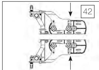
43. **Forward/Aft-**Loosen knobs underneath foot plates, slide foot plates into position. Tighten knobs securely
