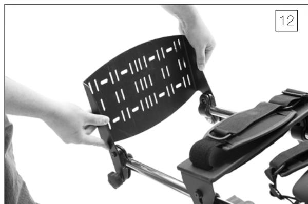
13. If the multi-adjustable foot plates were ordered, place each foot plate onto the legs. Tighten knobs securely.
