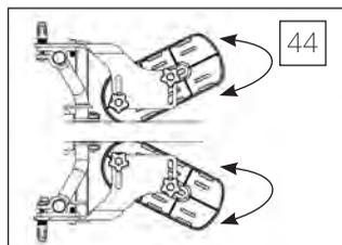
45. **Abduction-**Loosen ratchet handles to spread apart foot plates, tighten securely. Loosen knobs under foot plates and slide foot plates apart. Tighten knobs securely
