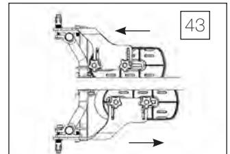
44. **Toe-in/Toe-out-**Loosen knobs underneath foot plates, slide foot plates into position. Tighten knobs securely
