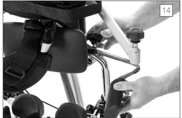
15. If the lateral supports were ordered, insert lateral supports into the bracket behind the upper body support pad. Tighten securely.
