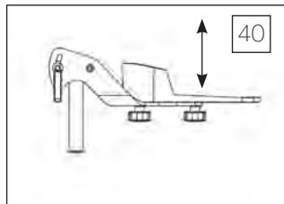
41. **Plantar/Dorsi-**Loosen ratchet handles to tilt foot plates. Tighten securely.
