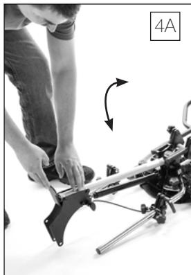
4B. Allow the mast post to come up to a vertical position.
