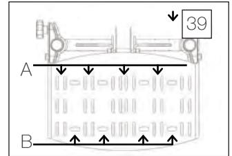
39B. **Foot Holders-**Position foot holders into desired position. Insert bolt and tighten knob securely.
