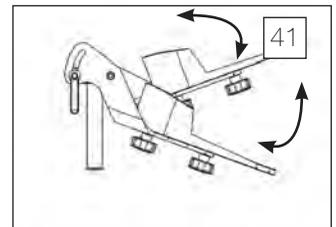
42. **Adduction-**Loosen knobs to slide foot plates together. Tighten knobs securely
