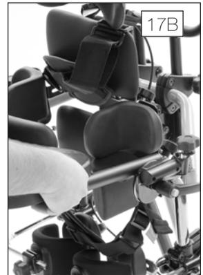
18. Remove head support and place the stem into the clamp as shown. Tighten securely.
