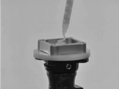
Check height measurement to ensure height is identical to test socket. Fill connector with glue.
