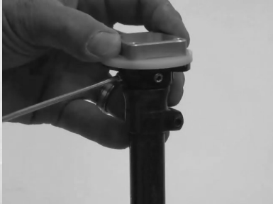
Attach pyramid to endo components. All components should be at neutral. Return mold and lock to alignment fixture.
