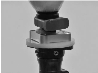
Lower mold and lock onto connector. Allow glue to set.
