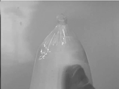
Pull PVA bag over cast. Use heat to help ensure PVA fits under lock funnel.
