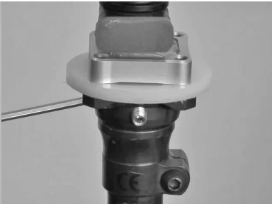
Remove mold (with lock and connector) from fixture.
