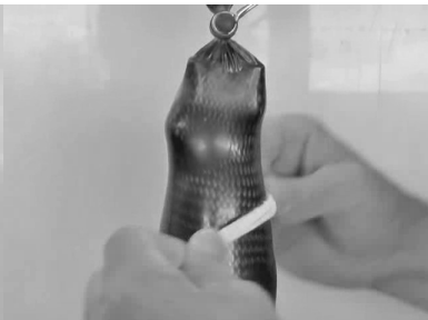
Pull outer PVA bag over mold. Laminate in customary fashion.
