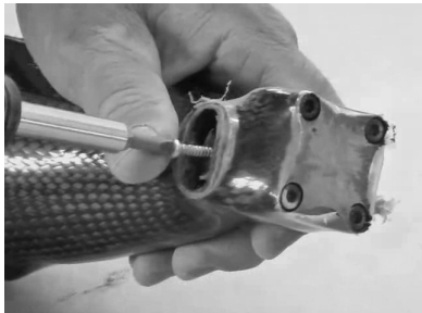
Remove foam rectangle and red silicone caps. Install removal screw in lamination tool. Remove lamination tool
