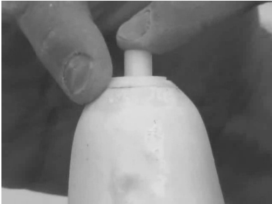
Glue anchor to cast. Fill in any gap with plaster and smooth transition. Mark location of release button.
