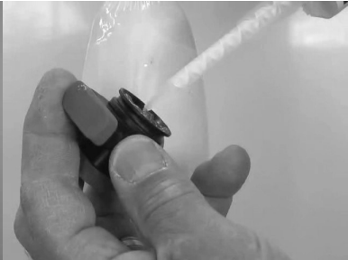
Apply a bead of glue to housing funnel and glue to anchor with lamination tool aligned with release button location mark.
