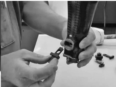
Slide lock plate into face plate and install spring.
