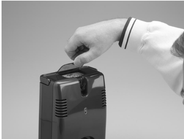
Figure 23: Lifting Dust Cover on Keypad Display
