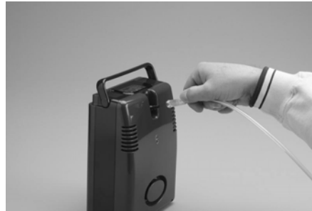
Figure 9: Connecting Cannula to FreeStyle's Oxygen Outlet
