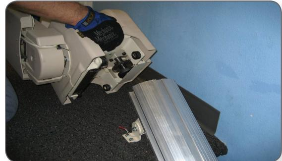
**Step 1:** Place the four track wheels onto the fixed axles at the front and rear of the chassis. The white surface on the rollers should face the axle on the chassis.
