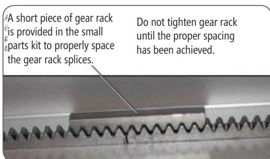
**Step 3:** When the gear rack is timed, use the 9/64" Allen wrench to tighten the gear into place.
