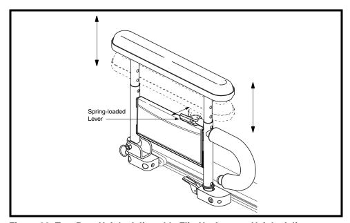
Figure 30. Two Post Height Adjustable Flip-Up Armrest Height Adjustment
