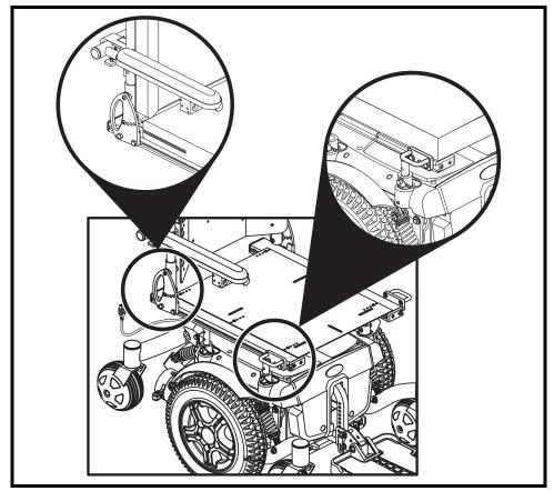
Figure 2. Unoccupied Securement Brackets on a Synergy Seat
