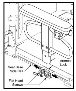
Figure 22. Heavy Duty Drop-In Armrest Position Adjustment
