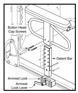
Figure 23. Heavy Duty Drop-In Armrest Height Adjustment
