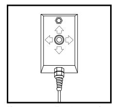
Figure 9. 4-way Toggle Operation
