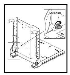
Figure 7. Flip-forward Back Canes (Latched)
