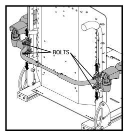
Figure 17. Height Adjustment for Figure 18. Height Adjustment for Cantilever Armrests Attached to the **Push Bar**
