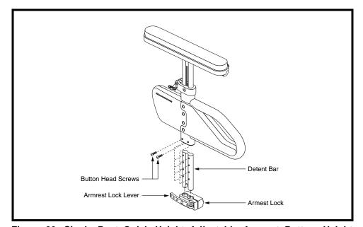
Figure 26. Single Post Quick Height Adjustable Armrest Bottom Height Adjustment
