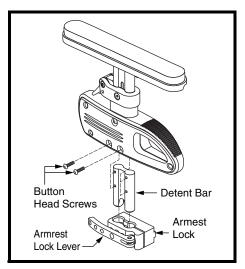
Figure 28. Pediatric Single Post Quick Height Adjustable Armrest Bottom Height Adjustment
