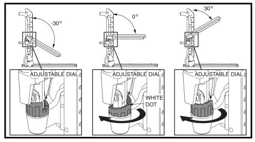
Figure 16. Cantilever Armrests Angle Adjustment
