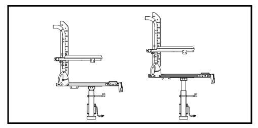
Figure 34. Power Seat Elevator Option on a Synergy Seat
