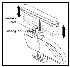
Figure 25. Single Post Quick Height Adjustable Armrest Top Height Adjustment
