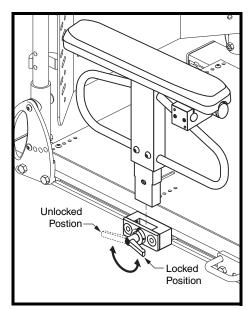
Figure 21. Heavy Duty Drop-In Armrest Removal/Installation
