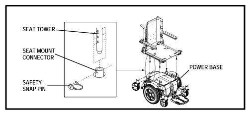
Figure 3. Seat Installation/Removal
