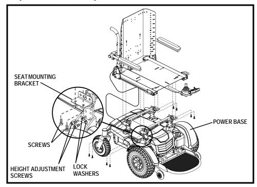
Figure 5. Seat Installation/Removal on Quantum/Jazzy 1450
