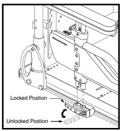
Figure 24. Single Post Quick Height Adjustable Armrest Removal/Installation
