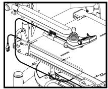
Figure 33. Controller Harness Routing
