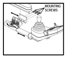
Figure 31. Controller Position – Depth
