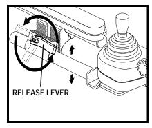
Figure 32. Controller Position – Height
