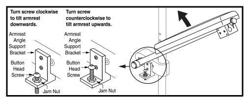
Figure 19. Flip-Up Armrest Angle Adjustment
