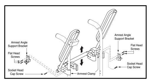
Figure 20. Flip-Up Armrest Height Adjustment
