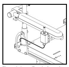
Figure 8. 2-way Toggle Operation
