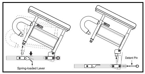
Figure 29. Two Post Height Adjustable Flip-Up Armrest Removal and Installation
