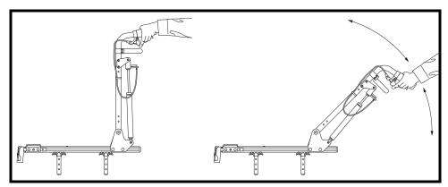
Figure 36. Manual Recline Angle Adjustment
