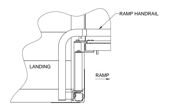
PLATFORM HANDRAIL TERMINATION DETAIL SCALE 1:3
